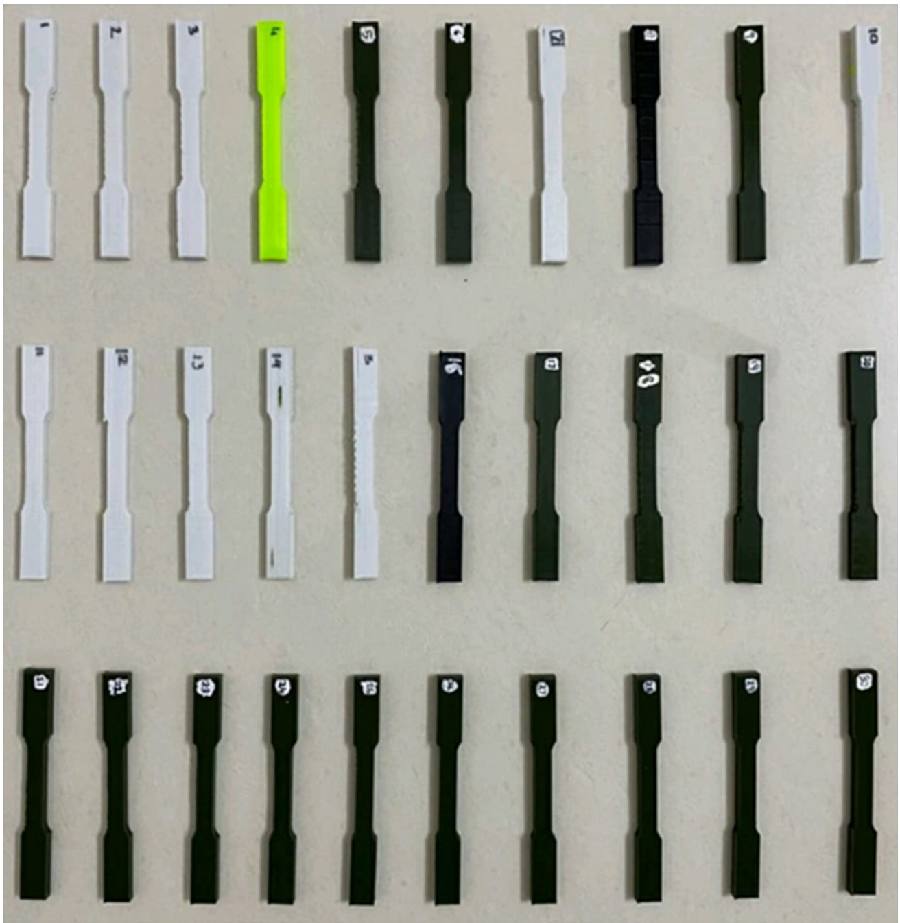
Figure 1 Additive manufactured PLA specimens
