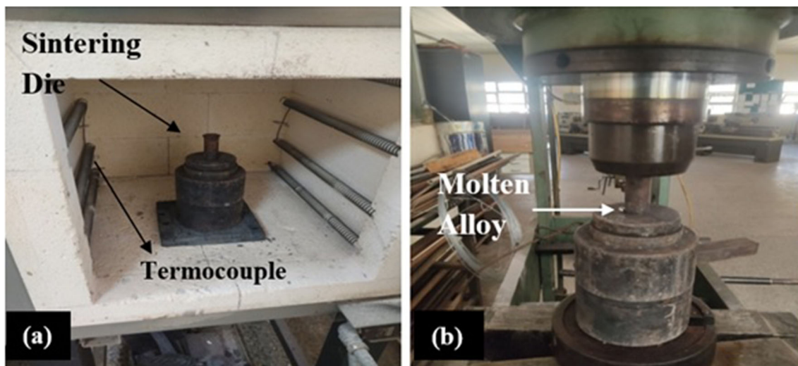
Fig. 2 (a) Sintering of Al-xCu alloys in the die and (b) pressure application after sintering.
