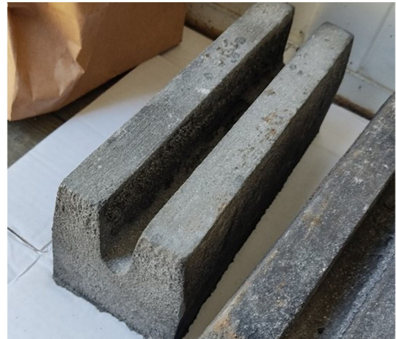
Fig. 1 The shape of the cast bloc of high-chromium cast iron before cutting and machining: (a) schematic from the DIN 1563:2012-03 standard where the cross-hatched zone is the one to be extracted for sample extraction. (b) A cast bloc before machining
