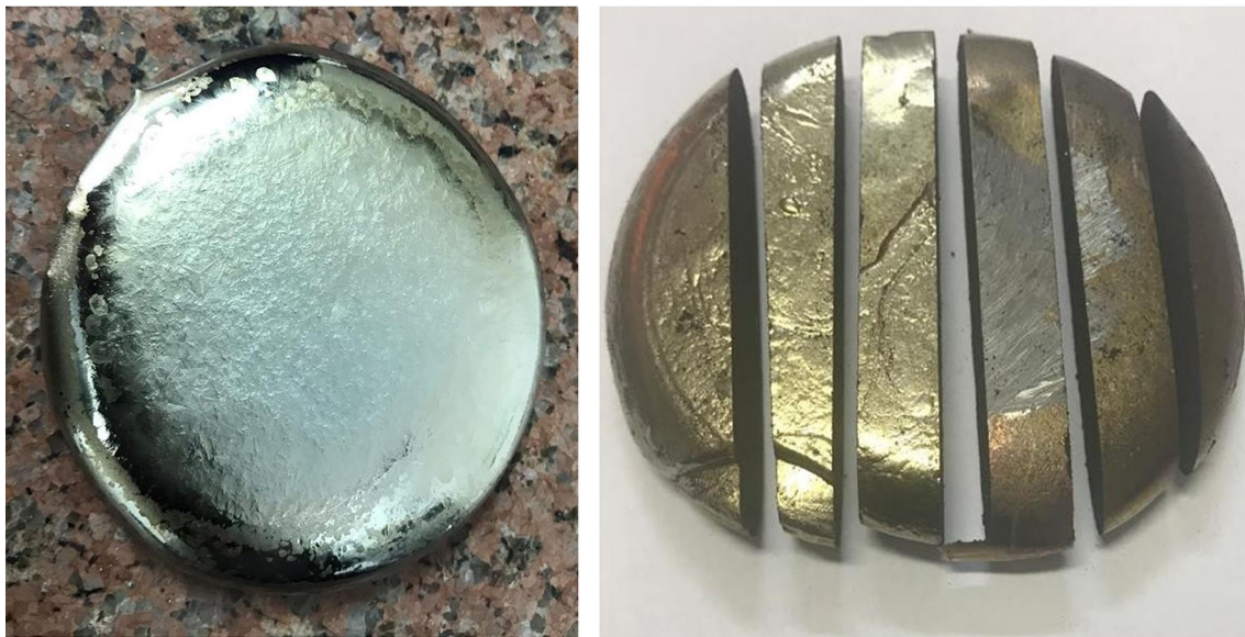
Fig. 2 Shape of alloy ingots (disk shape \Phi 80 \times 10 mm)
