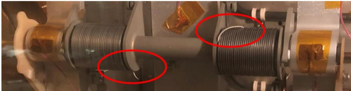
**Fig. 3** Image of spring mechanism during thermal testing with hardware failure circled
