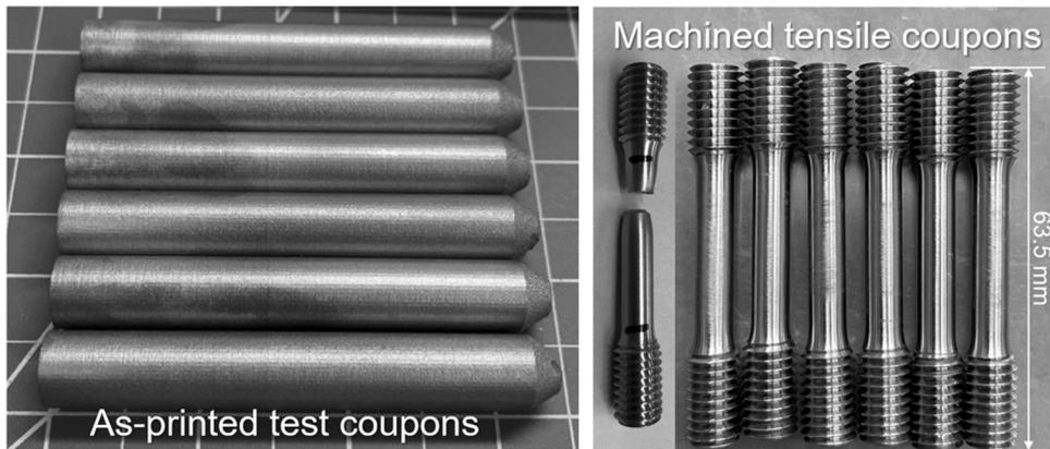
**Fig. 9** Tensile coupons shown as printed and after machining
