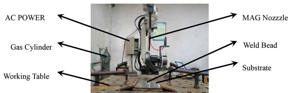
Fig. 1 Experimental platform for wire and arc additive manufacturing
