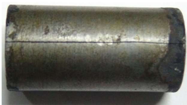
Fig. 21. Quench crack observed in AISI 52100 steel while quenching in distilled water and carbonated water. Reprinted by permission from Springer Nature Customer Service Centre GmbH: Springer Nature, Transactions of the Indian Institute of Metals , Comparison of Cooling Behaviour of Carbon Steels in Polymer, Oil and Carbonated Quench Media, N.G. Mathews, K.M.P. Rao, U.V. Nayak, K.N. Prabhu, Copyright 2019 [95]
