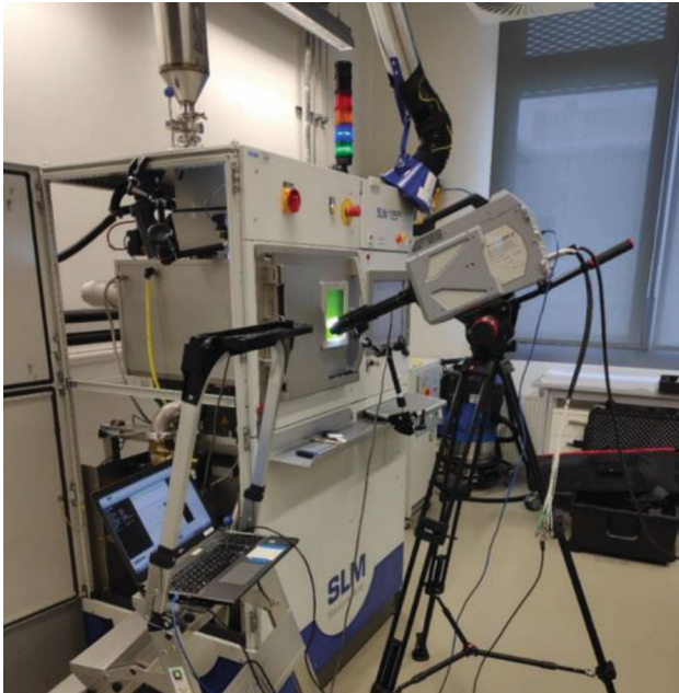
Fig. 3 SLM@125HL and high-speed camera setup
