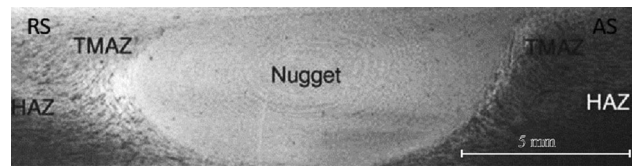
Fig. 7 Cross-sectional plane of welded joint showing various zones of square pin friction stir-welded AA2024
