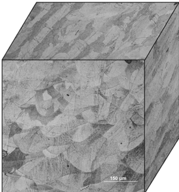
Fig. 1 A typical bulk-build structure, viewed on three section planes. The top surface is normal to the beam ( z axis) and parallel to the scan ( x - y ) plane. Laser scan directions within the scan plane include the direction normal to the front face along with 60 and 120 degree rotations about the z axis from the front face normal.
