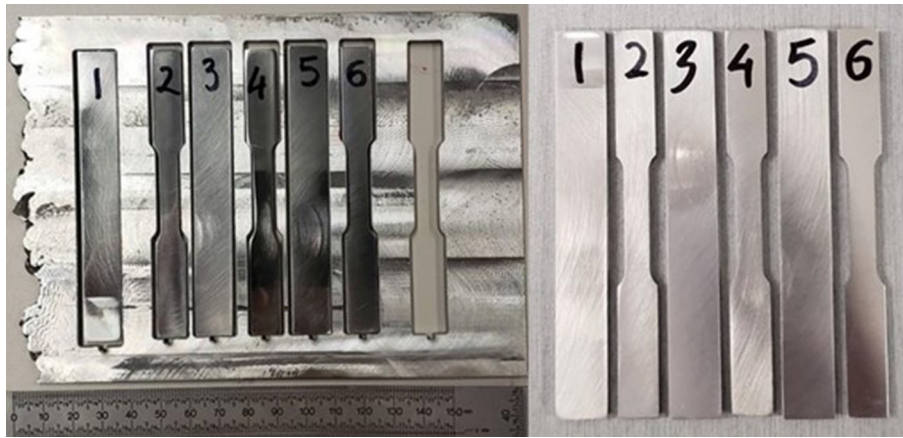
Fig. 5 Removal of bend test samples (#1, #3, and #5), dimensions: 100 mm high, 12.5 mm wide, 2.5 mm thick; and tension test samples (#2, #4, and #6), dimensions: 100 mm high, 10 mm wide, 2.5 mm thick, R = 6 mm, gage length: 25 mm high, 6 mm wide; grip length: 30 mm high
