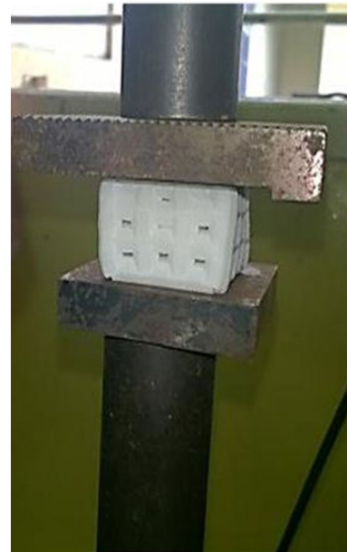
Fig. 8 Compression testing of scaffold
