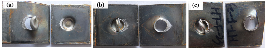
Fig. 14 Fatigue failure modes of clinched joints after local heat treatment
