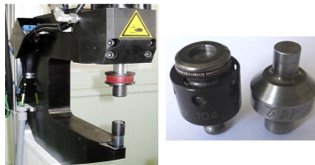
Fig. 2 Clinching machine and cycle extensible die clinching tools
