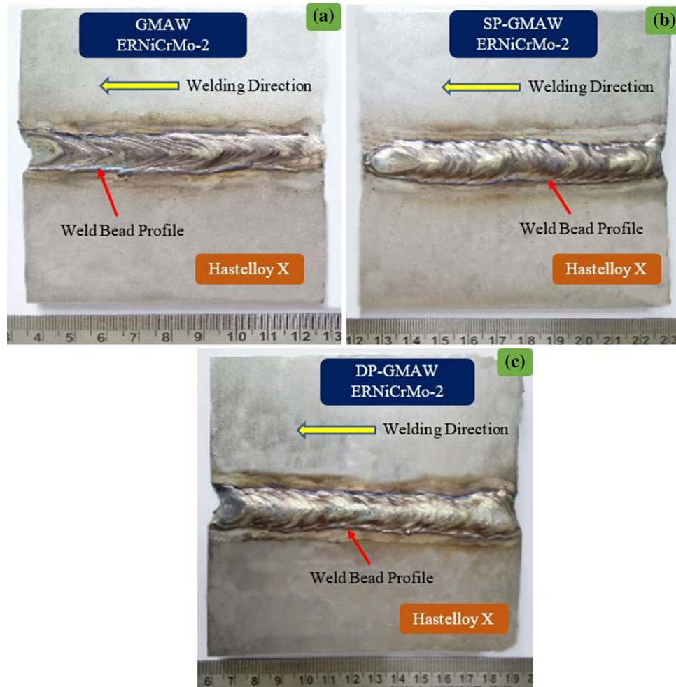
Fig. 1 Hastelloy X welded by (a) GMAW-ERNiCrMo-2 (b) SP-GMAW-ERNiCrMo-2 (c) DP-GMAW-ERNiCrMo-2
