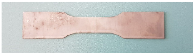
Fig. 3 Tensile test specimens and dimensions
