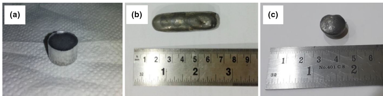
Fig. 1 (a) Cold-compacted pellet, (b) cylindrical shape, and (c) button shape of as-cast HEA samples
