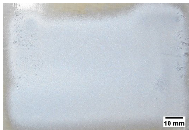
Fig. 6 Coating obtained through cold spray deposition. The sample depicted is the coating with 45% Al 2 O 3 content
