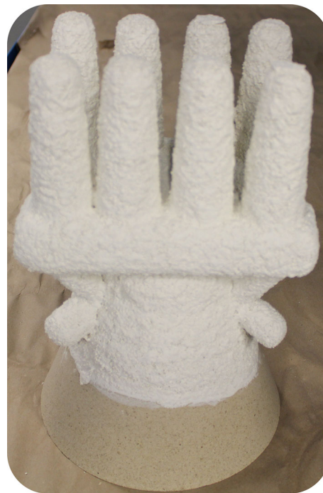
Fig. 1 Shell mold fabricated through the “dip and stucco” technique
