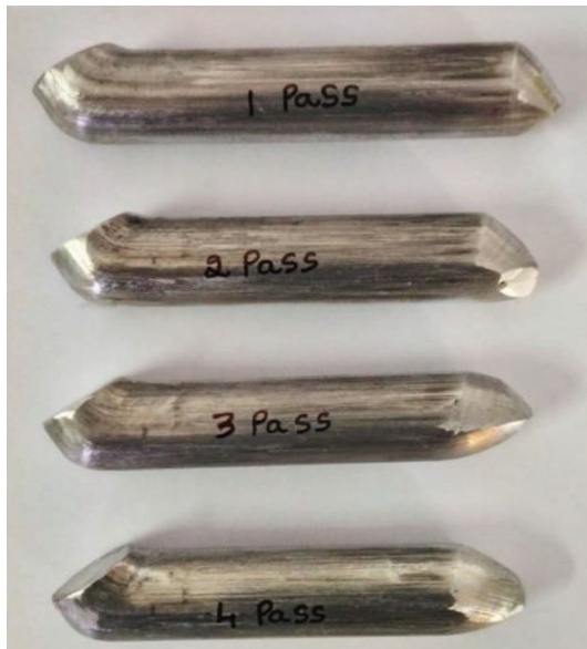
Fig. 4 Al-5Zn-2Mg alloy ECAP processed up to four number of passes at 150 °C
