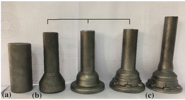
Fig. 1 Combined forging process of a flange shaft. (a) Billet, (b) three-stage hot forging, (c) cold ironing
