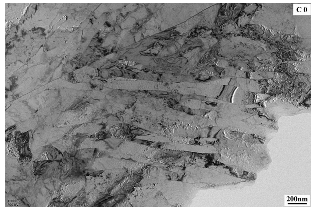
Fig. 6 The morphology of martensite lath of the 0Cr12Mn5Ni4-Mo3Al steel
