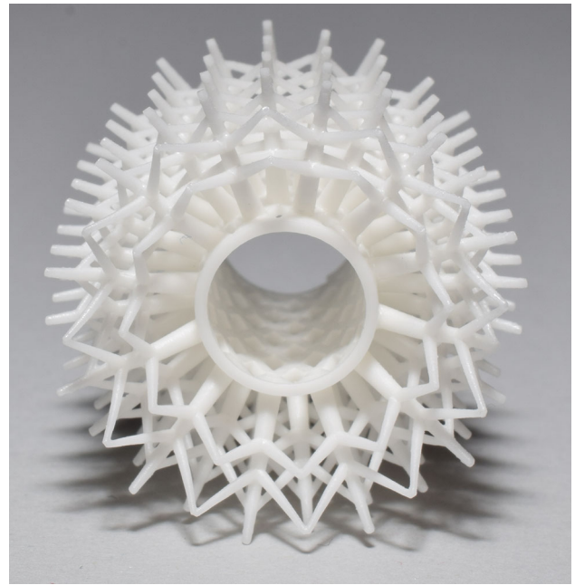
Fig. 7 Heat exchanger—sample 5—pipe with complex AM structure; defect-free sintered alumina component—top view
