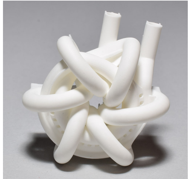
Fig. 10 Heat exchanger—sample 7—alternative heat exchanger structure; defect-free sintered alumina component; top view
