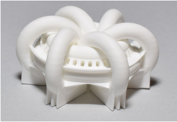
Fig. 9 Heat exchanger—sample 7—alternative heat exchanger structure; defect-free sintered alumina component
