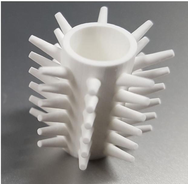
Fig. 5 Heat exchanger—sample 4—pipe with frustums instead of ribs; defect-free sintered alumina component
