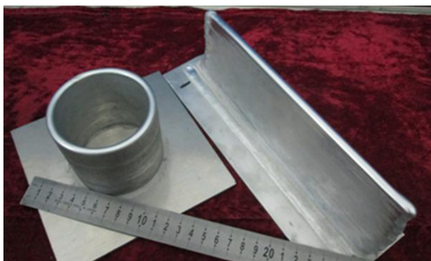
Fig. 1 GTA-additive manufactured 2219-Al parts
