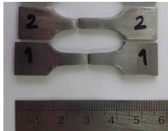
Fig. 9 Fracture locations for the tensile tested specimens (1: BM, 2: welded sample)
