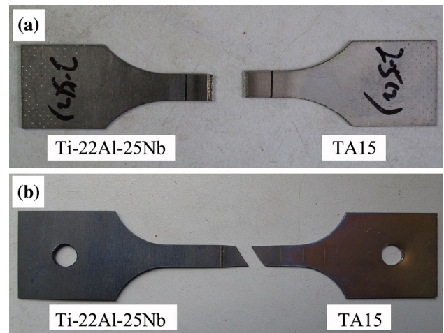
Fig. 15 Typical photograph of butt-welded joints after tensile testing at (a) room temperature and (b) 550 °C
