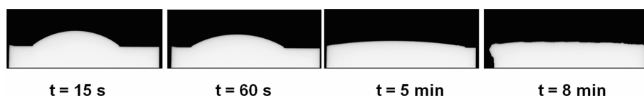
Fig. 13 Wetting sequence of NiB17 on \text{HfB}_2 at 1130^\circ\text{C}
