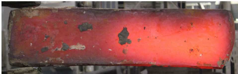
Fig. 16 The thick plate of Ti-35V-15Cr-0.3Si-0.1C forged using the optimized parameters
