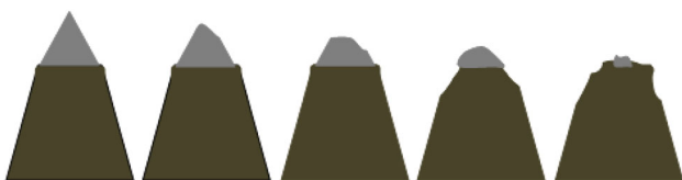
Fig. 3 Sketch of gradual wearing of conical picks used in continuous miner machine
