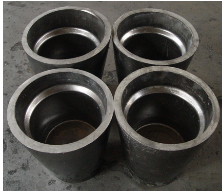
Fig. 11 Four successful Mg-13Gd-4Y-2Zn-0.6Zr alloy components
