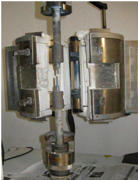
Fig. 1 Hot tensile testing apparatus and fractured specimen
