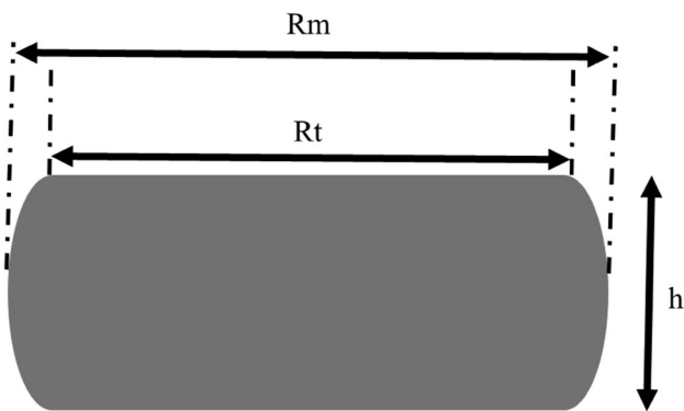
Fig. 3 Schematic figure of the specimen shape change after hot compression process
