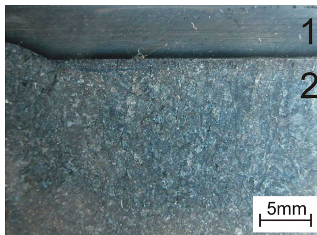
Fig. 3 Example transverse section of the bimetallic casting: 1—working layer in the form of alloy steel X2CrNi 18-9 plate, 2—base part of unalloyed cast steel at a carbon concentration equal to 0.60 wt.% and a pouring temperature of 1650 °C
