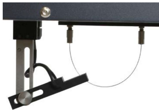
Fig. 11 Alternate break sensor to eliminate edge burnishing
