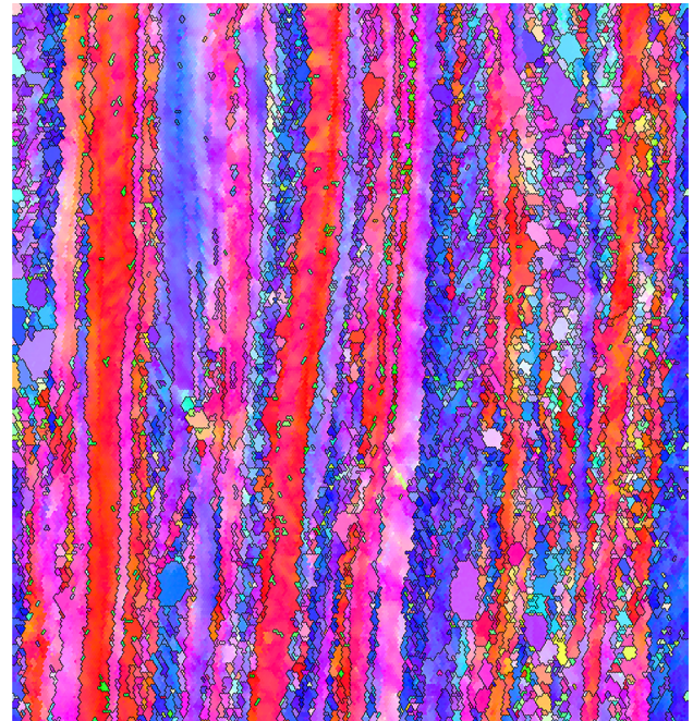
Fig. 5 Orientation map and constant \phi ODF sections for Ti-IF steel sheet annealed for 10 s
