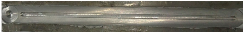
Fig. 2 Upper surface of groove cut on the FSPed zone
