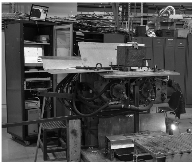
Fig. 2 Twin-roll caster used for the experimental program
