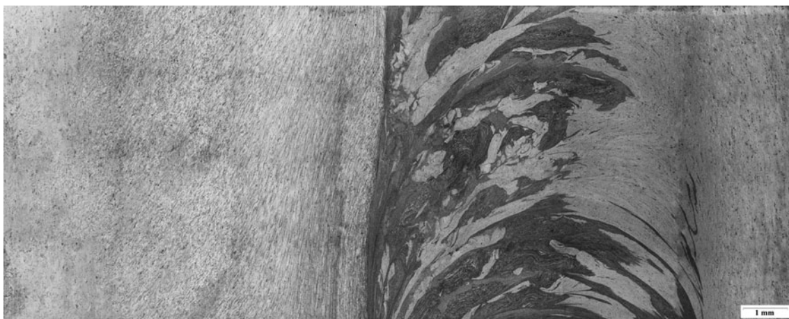
Fig. 4 Macrostructure of L4 layer of the weld—4.0 mm from the face of the weld
