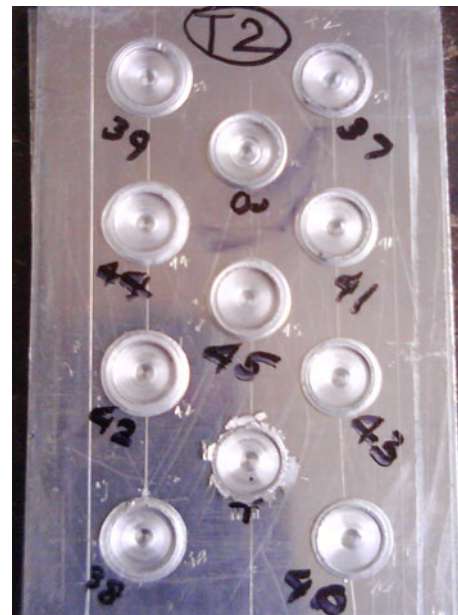
Fig. 4 Spot welds produced using Tool # 2 by various process parameter combinations
