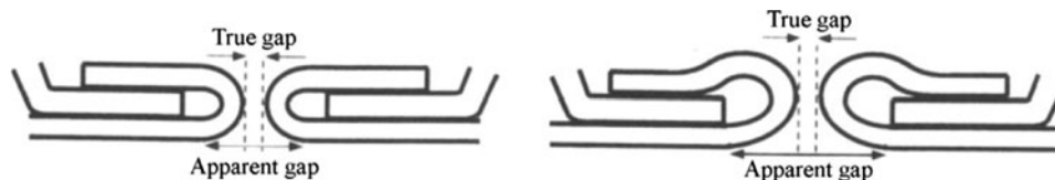
Fig. 3 Visual quality differences of hem unions—“flat-hemming” union used with steels (left) and “rope-hemming” union used with low formability alloys (right) (Ref 4)
