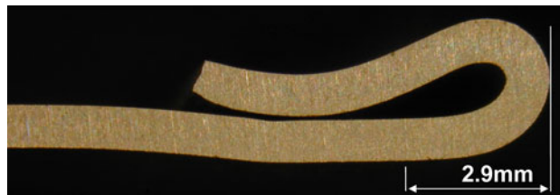
Fig. 11 Cross-sectional view after EM hemming with 7.20 kJ energy input (roll-in: 0.73 mm; hem union radius: 2.9 mm)
