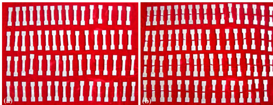
Fig. 3 Tensile specimens. (a) Before and (b) after tensile test
