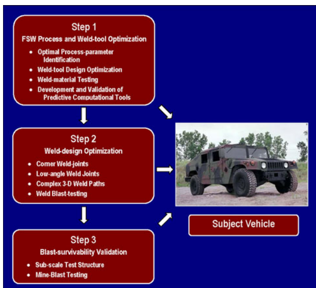
Fig. 18 A three-step procedure for the introduction of friction stir welding (FSW) technology and high-strength age-hardened aluminum alloys to the construction of blast-survivable military-vehicle underbody hull structures
