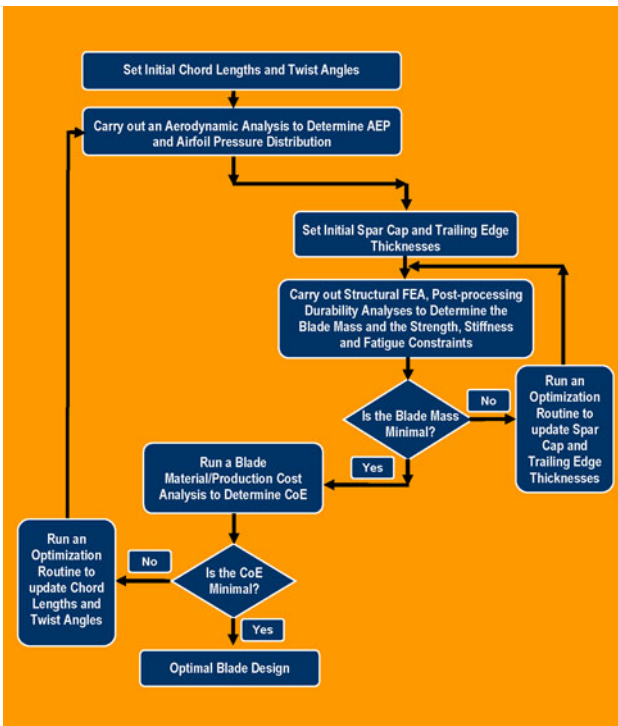
Fig. 5 A flow chart for the two-level multidisciplinary design optimization procedure for cost-effective 5 MW HAWT blade developed in the present work
