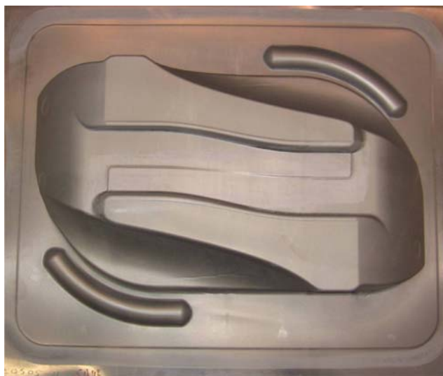
Fig. 9 A photograph of a fully formed panel using the CSPF process
