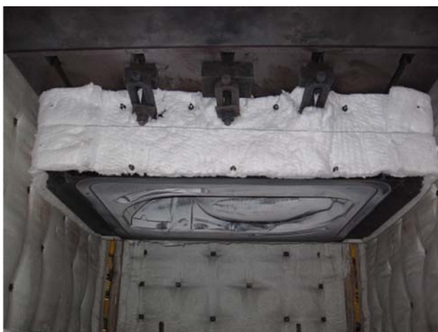
Fig. 4 Photograph of the CSPF die cavity for forming the panel
