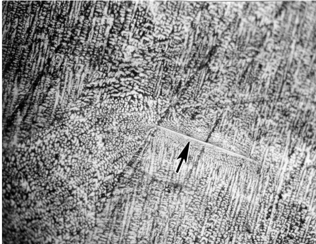
Fig. 1. Rod-like intermetallics of Ag_3Sn in the matrix of Sn. Annealing for 100 h at 373K. Optical microscopy, x160.
