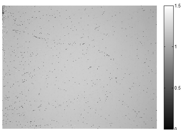
Fig. 11 Thermal response pixel mapping attained for a 293 K black-body screen illumination for a MWIR HgCdTe FPA operated at 77 K.
