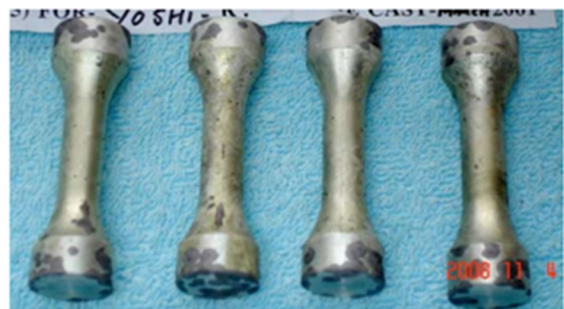
Fig. 7 Tin pest allotropic transformation on Sn-0.5Cu bulk solder samples, reprinted with permission from Plumbridge. 17
