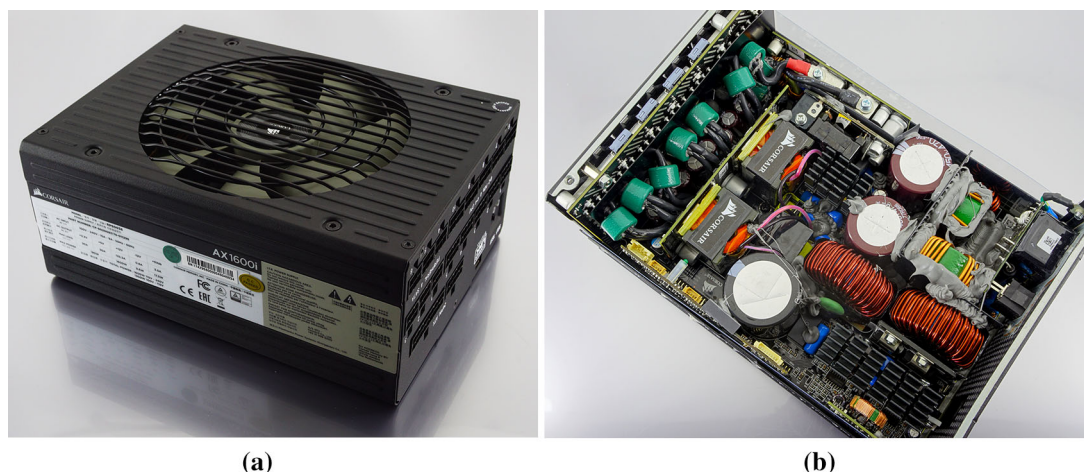
Fig. 16. External (a) and internal (b) view of Corsair 1600 W GaN-based computer PSU (Model: AX1600i) © 2020 EnVeritas Group. Reprinted, with permission
