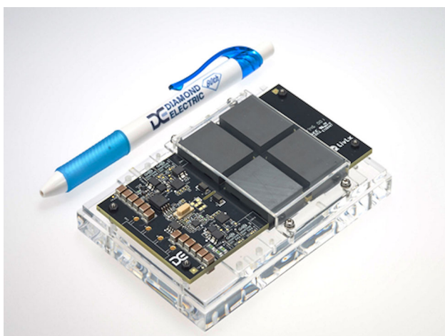
Fig. 7. GaN-based 1 kW isolated bidirectional DC–DC converter developed by Diamond Electric Mfg. Co. © 2020 Power Electronics World™. Reprinted with permission
