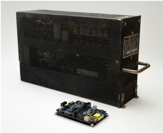
Fig. 10. Comparison between Aveox's GaN (compact) and silicon-based (large) power conversion systems highlighting the significant improvement in power density using GaN semiconductors © 2020 GlobeNewswire. Reprinted with permission
