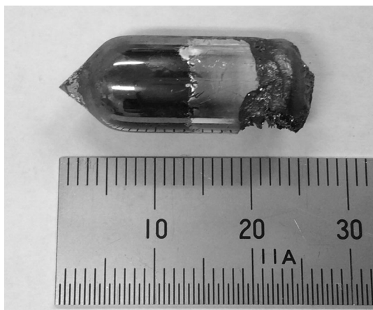
Fig. 1. Example of the resulting CdTe 0.5 Se 0.5 ingot grown by Cd solution.
