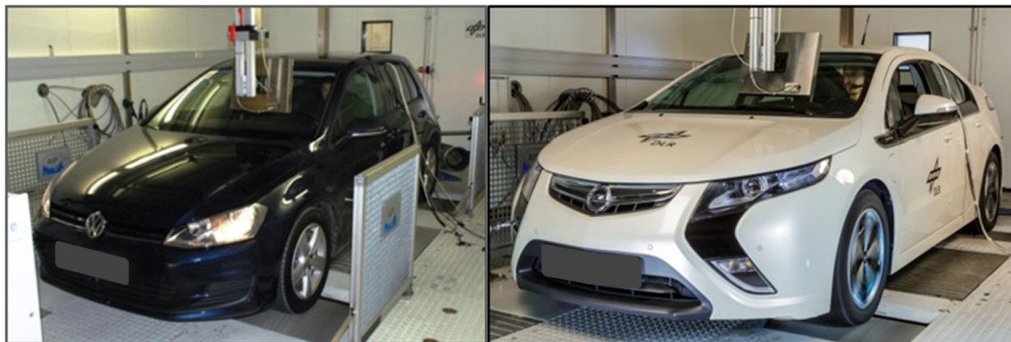
Fig. 10. Reference vehicles at the roller dynamometer test bench. 16
