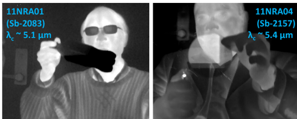
Fig. 6. FPA images ( 320 \times 256 ) at 150 K from two different MWIR InAs/InAsSb superlattice nBn samples.
